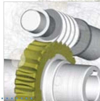
In order to increase silence, efficiency and duration, the wormshaft is made in case hardened steel and ground machined, while the worm wheel is in shell cast ZCuSn12 bronze.
