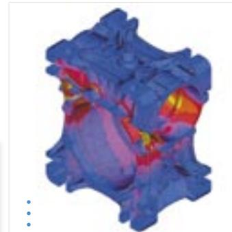
The housing has been designed with parametric three-dimensional CAD SW supported by programs of analysis of the thermal dissipation capacity and the structural resistance/deformation under the effect of working loads.
